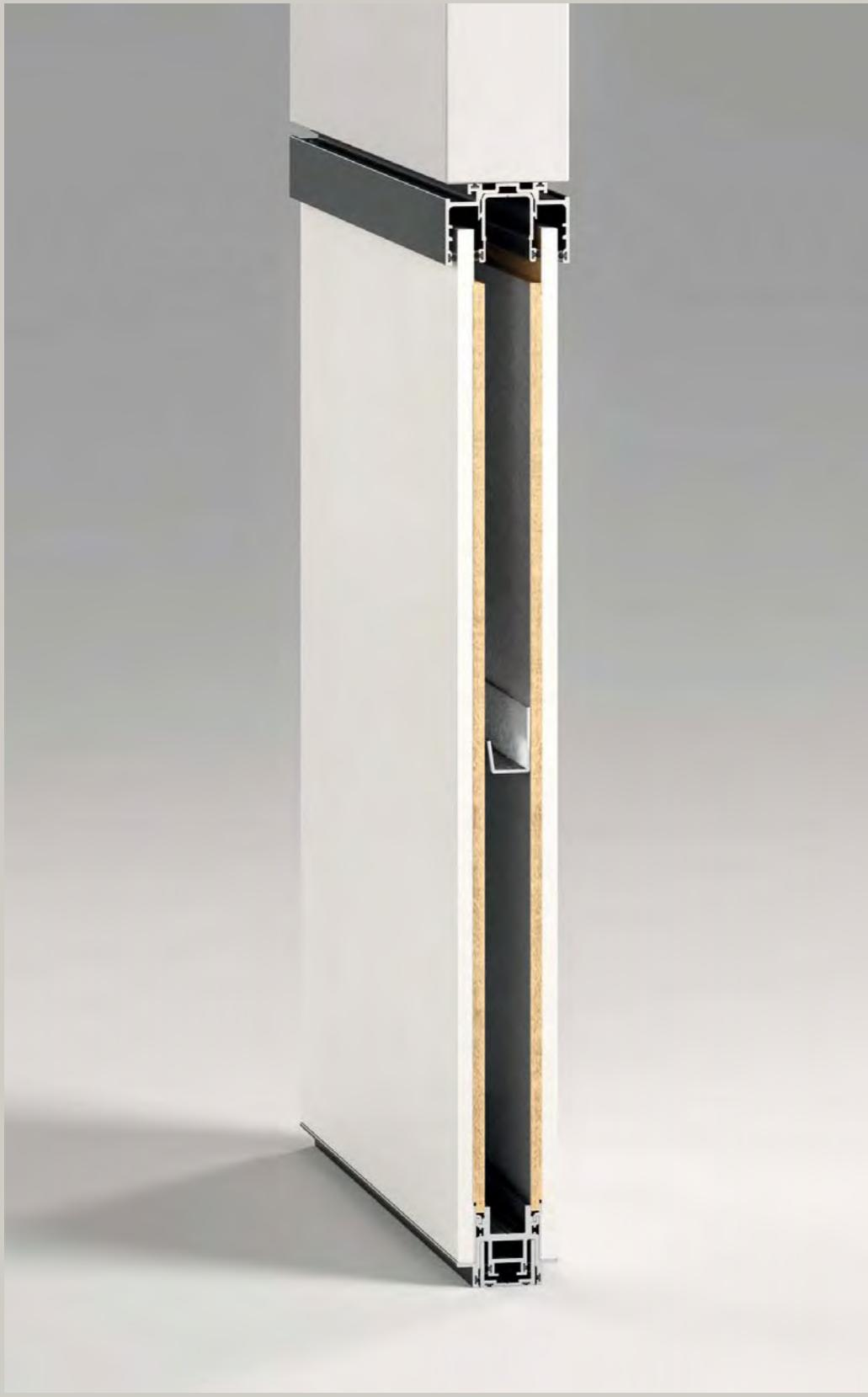
**The solid wall is made with 18 mm thick melamine-faced chipboard, shaped to the aluminium frame. The cavity between the panels can be filled with soundproof insulation. The frame is similar to the glazed version, with aluminium profiles and gaskets that help to dampen noise and aid stability.**
